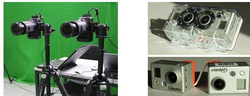
Figure 10: The set-ups used in our experiments. From left to right: A pair of Canon EOS 550D cameras, the GoPro 3D Hero system.
