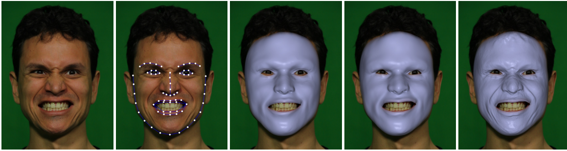
Figure 2: Algorithm overview: Left to right: (a) Input video frame, (b) sparse feature tracking (Sec. 5), (c) expression and pose estimation using a blend shape model (Sec. 6), (d) dense expression and pose correction (Sec. 7), (e) shape refinement (Sec. 8).
