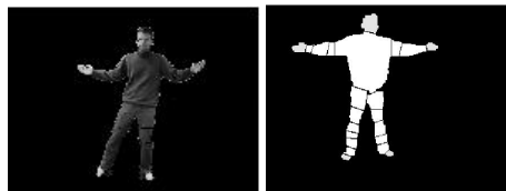
Figure 2: Video frame after background subtraction (l). GVD segmentation of silhouette in initialization position (r)
