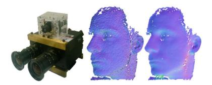
**Figure 26.2:** Left: our active stereo sensor. Middle: patch-match result. Right: Result after variational refinement.
