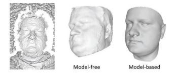
**Figure 10.1:** Comparison: Model-free approaches (Kinect Fusion,  $256^3$  voxel grid) are prone to oversmoothing. In contrast to this, our model-based approach allows to estimate fine-scale surface details.
