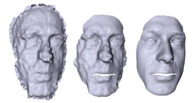
**Figure 6.4:** Generic face fitting: (from left to right) input scan, registered average face and best fitting morphable model.
