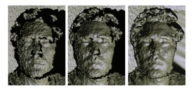
Figure 6.2: Data preprocessing: Left: raw data from a single frame. Middle: temporally smoothed data. Right: additionally Gauss-filtered data
