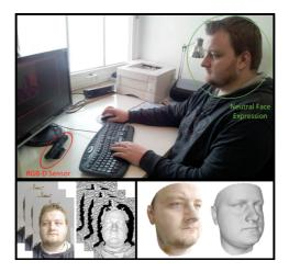
**Figure 9.1:** Hardware setup: The RGB-D stream of a single PrimeSense Carmine is used to reconstruct high-quality head models using an interactive and intuitive reconstruction paradigm.
