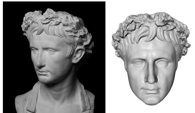
Fig. 7: Digitized Statue: We reconstruct the 3D-Geometry of the statue on the left side using structured light scanning.
