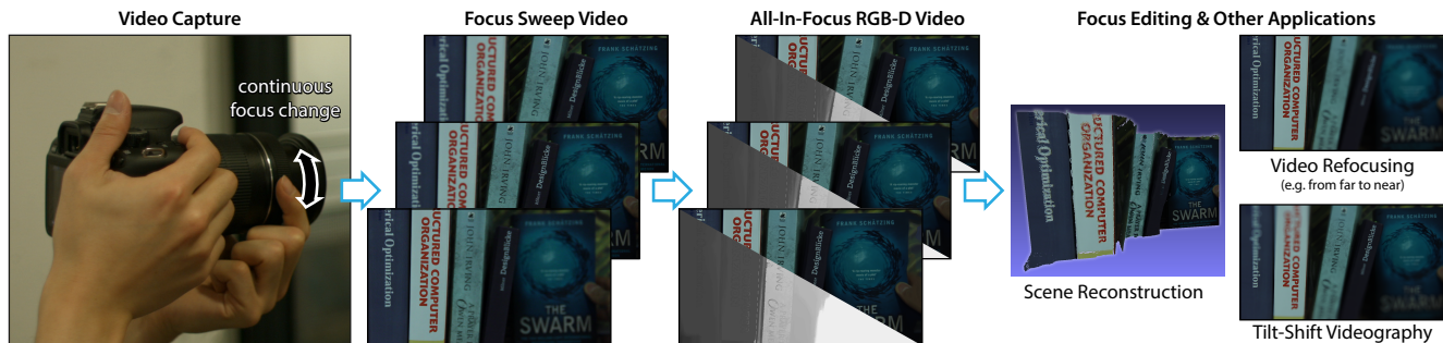
Figure 1. We capture focus sweep videos by continuously moving the focus plane across a scene, and then estimate per-frame all-in-focus RGB-D videos . This enables a wide range of video editing applications, in particular video refocusing. Please refer to the paper’s electronic version and supplemental video to more clearly see the defocus effects we show in our paper.
