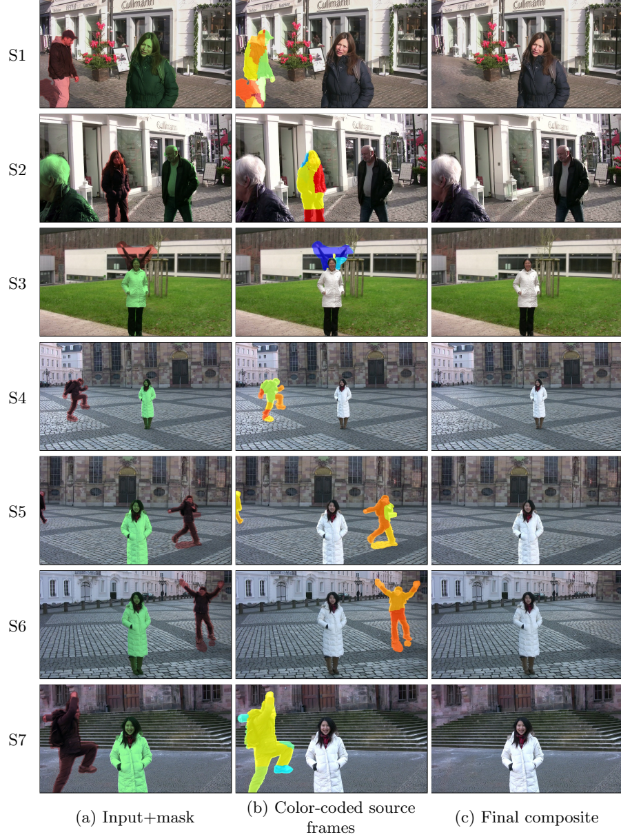
Fig. 6. Results of inpainting in our seven test sequences: (a) an input frame and overlaid masks for the hole and dynamic objects (shaded in red and green, respectively); (b) visualization of the source frames obtained by minimizing Eq. (5); (c) inpainting after compositing and gradient domain fusion. Subjects in S3-S7 were kindly provided by the Ministry of Silly Walks.
